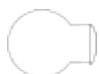
Symbol for a profile on a lighting plan (derived from the shape of early profiles, like the Pattern 23 above)
