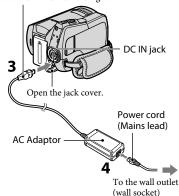
You can charge the "InfoLITHIUM" battery pack (H series) after attaching it to your camcorder.
