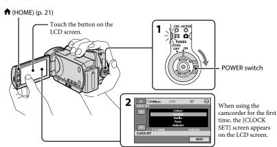
While pressing the green button, turn the POWER switch repeatedly in the direction of the arrow until the respective lamp lights up.
